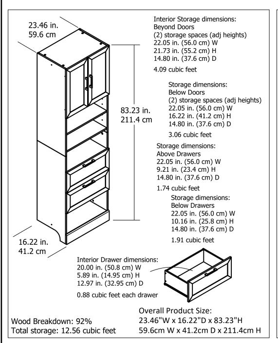
Adjustable Shelf hole spacing: 2.50 in. (6.4 cm) 30 lbs. / 13.6 kg. 0 lbs. (each adjustable shelf) 0 kg. 40 lbs. / 18.1 kg. (each fixed shelf) 20 lbs / 9.1 kg (each drawer) 40 lbs. 18.1 kg. **Maximum Weight Capacities** Unit Weight: 103 lbs. (46.7 kg)
